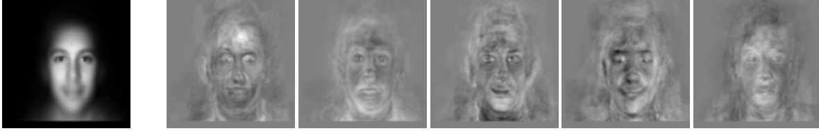
Figure 2. The average face and the first five eigenfaces for a sample 600 class training set.
